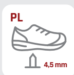
PL Durchtrittshemmung Textil (4,5 mm Nagel) Penetration Resistance Textile (Large Nail)
